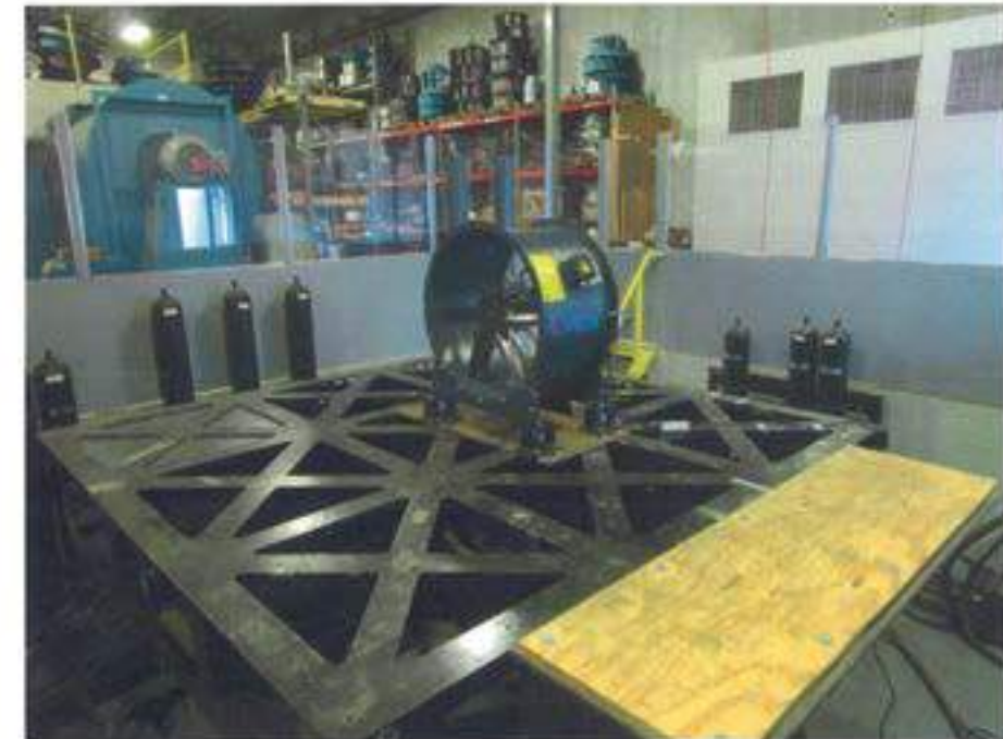
800mm Tubeaxial Seismic Test Setup
