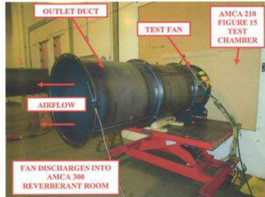
800mm Tubeaxial Air and Sound Test Setup
