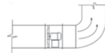
Appropriate duct design
