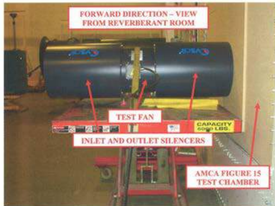
400mm Tubeaxial Air and Sound Test Setup
